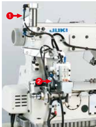
1 Presser lifter drive mechanism air cylinder 2 Thread trimmer drive mechanism air cylinder
