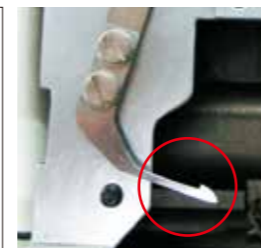
New cloth guide / The new cloth guide helps the machine perform hemming while keeping the hem width consistent.
