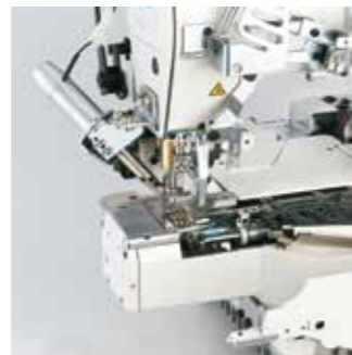
Electromagnetic needle thread / looper thread trimming device
